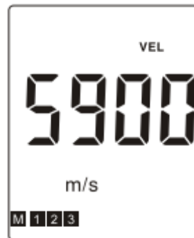
Last applied sound velocity & registered unit
